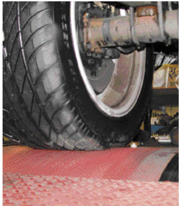
*A chassis dyno allows horsepower measurements to be made without having to remove the engine from the car. This is done by feeding torque into a set of rollers with the driven wheels. Chassis dynos are a precise and repeatable way to measure wheel horsepower.*
