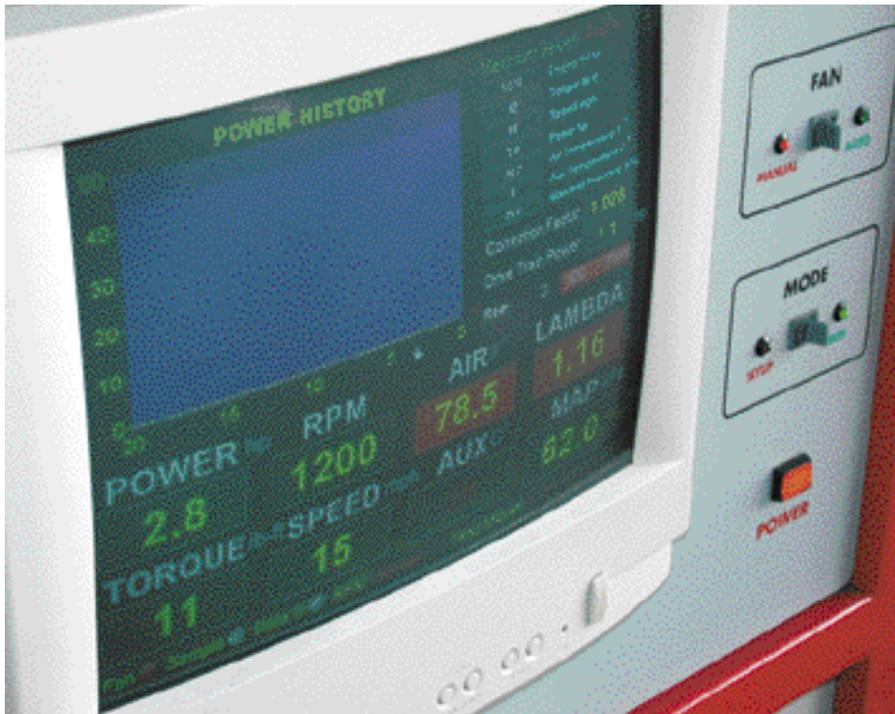
*Today's dynos are computer-controlled affairs. All of the calculations, including corrections for atmospheric conditions, are calculated by the machine.*
